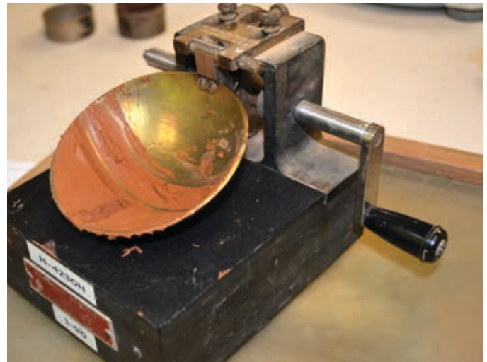
A device used for testing Atterberg limits, which is a method of testing the water content of different soil types.
