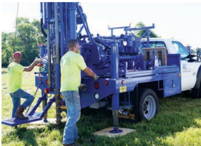
This truck-mounted drilling rig is one of the ways engineers may collect and test the soil at a construction site as part of a geotechnical investigation.
